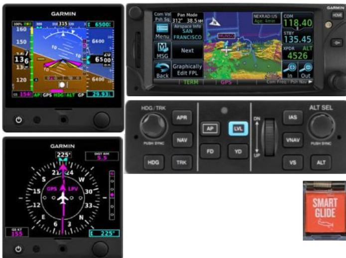
The Smart Glide feature is installed and accessible through menus in the GTN 650. The switch on the panel will be installed when the part is available. This feature hugely reduces the workload in an engine failure. It displays the closest reachable airports on the GTN 650 allowing you to choose, turns the plane in the direction of your choice and tunes the appropriate radio frequencies.
