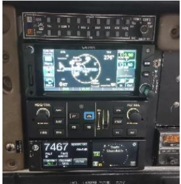
Our installation includes electric trim with the auto-trim feature. The included trim switch was deemed inadequate.. The shop saved us a ton of money, around \$900, by refurbishing our existing switch instead of buying a new upgraded switch and its mounting plate.
