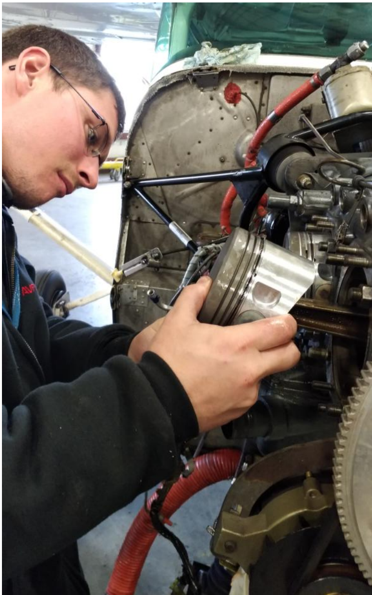
Mechanic Justin English installing a new piston.
