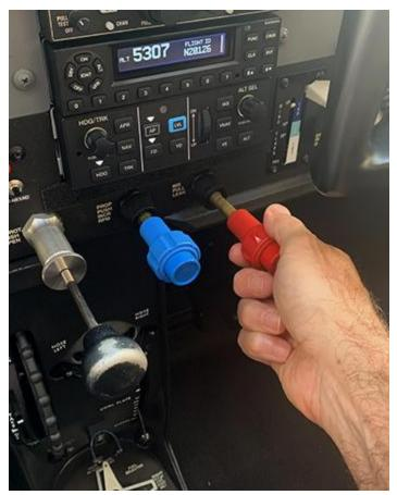
descend with cruise power, as many people do, the mixture getting leaner as you descend means you could create a power-mixture combination that's harmful to the engine. That means you should enrichen as you descend, erring on the side of being too rich. If you're unsure, just go full rich (or as needed for the highaltitude destination) early in the descent and be done with it. You'll burn more gas, but you'll have a high enough power setting that plug fouling shouldn't be an issue.
