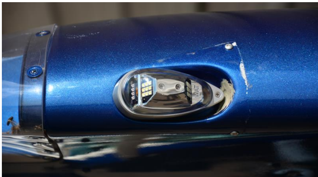
The Skyhawk's new left wingtip LED position / anti-collision light.
